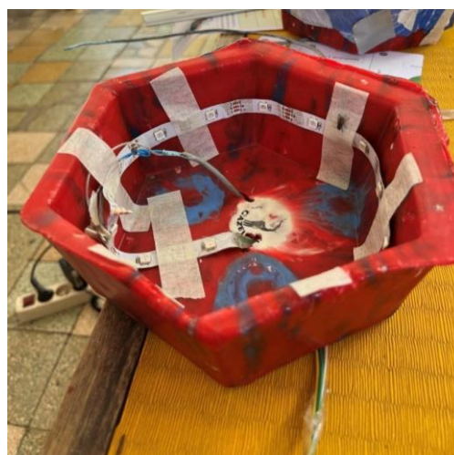
Gambar 8. Proses Perakitan Lampu Led Ws2812b
